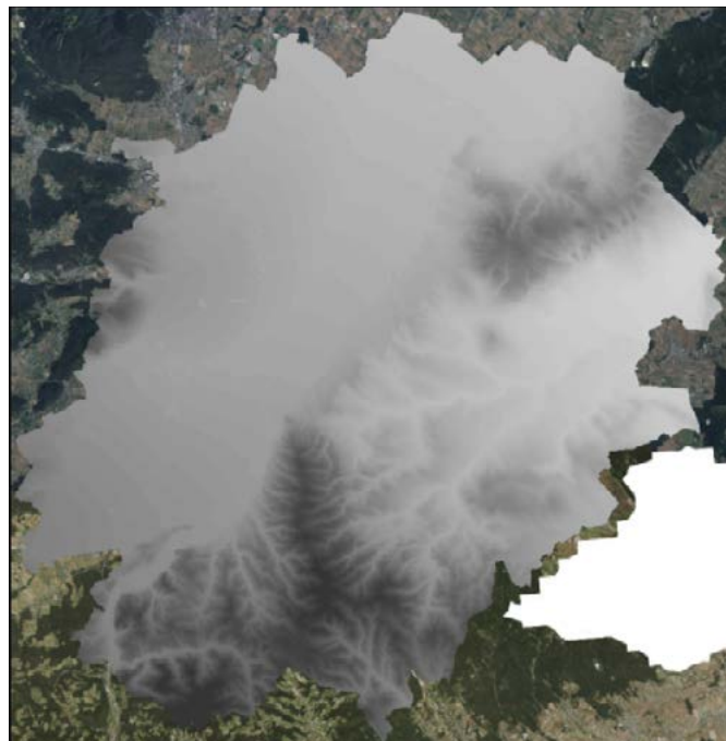
Figure 12: Layer “Digital Elevation Model” represents the ground elevation data of the terrain
